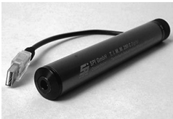
Fig. 6. An optical video microscope used for detecting fissures in wheel webs
